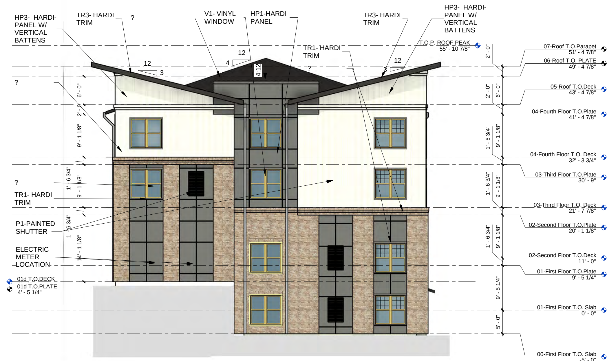
02 BUILDING 3 ELEVATION - MITCHELL RD. 3/32" = 1'-0"
