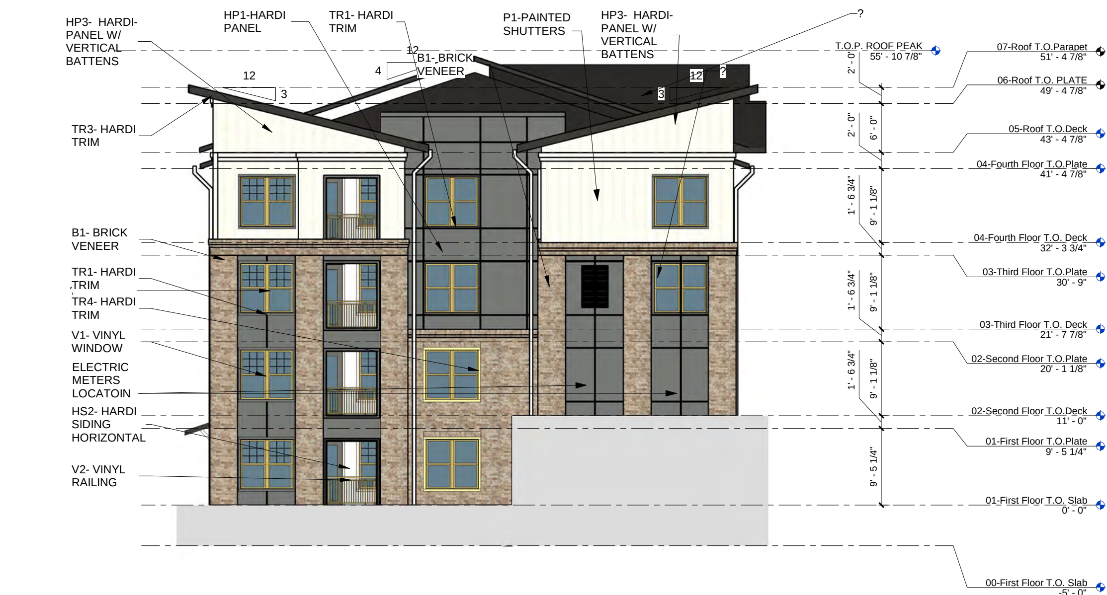
01 BUILDING 3 ELEVATION - ENTRY SIDE 3/32" = 1'-0"
