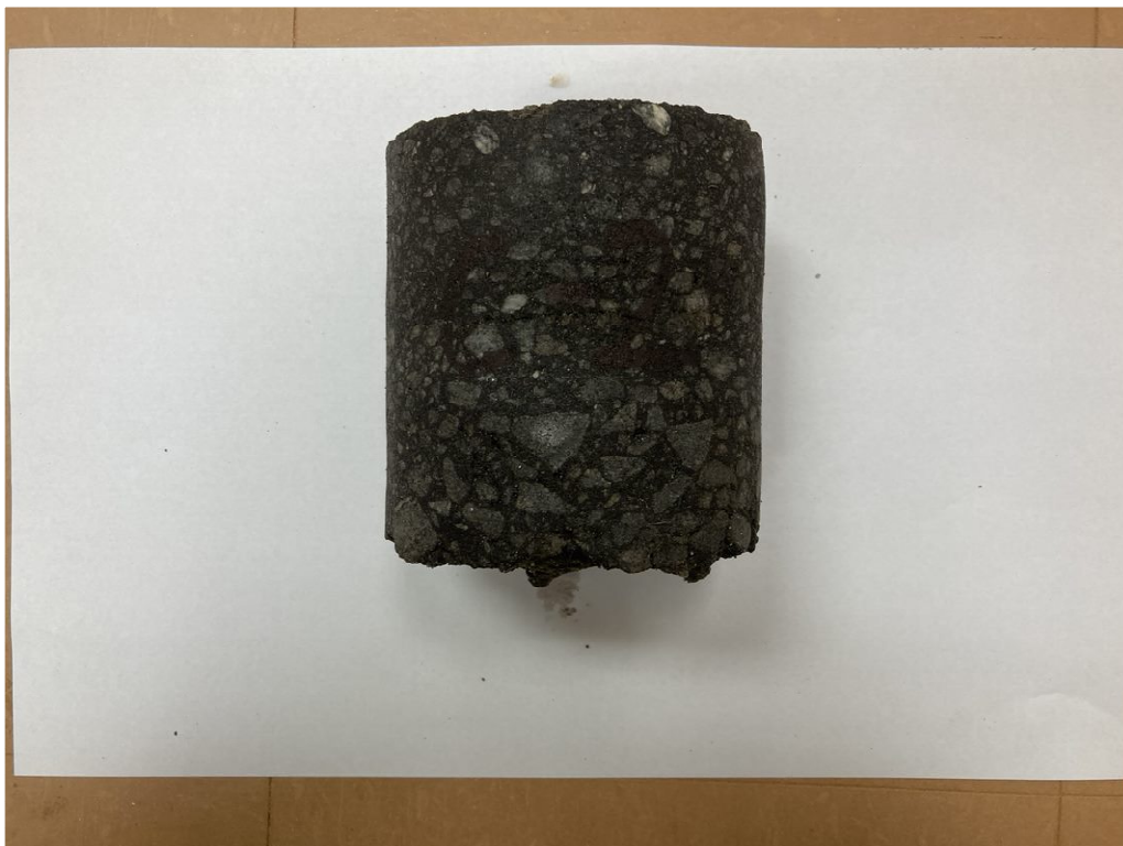
Photo 2. Core C-2. Asphalt Thickness = 5 inches
