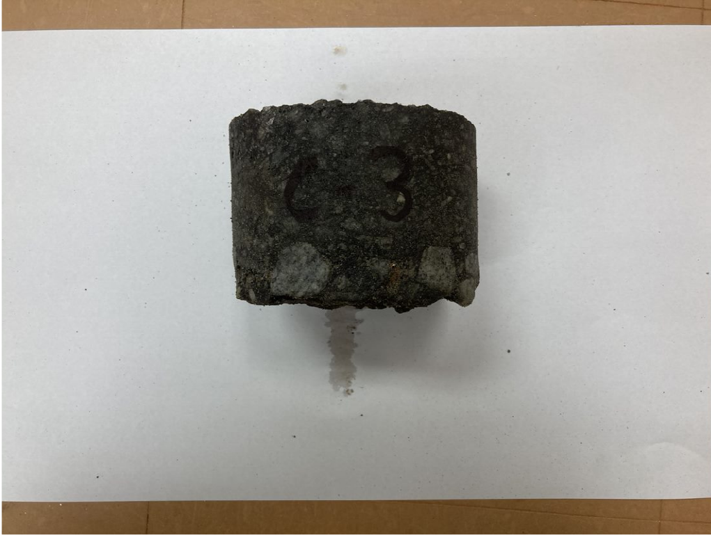
Photo 3. Core C-3. Asphalt Thickness = 3 inches
