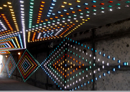
One approach to Suwanee's pedestrian tunnel project could be low tech, like this project that uses highway reflectors to illuminate a passageway. Richard Elliott, Thunder Over the Rockies
